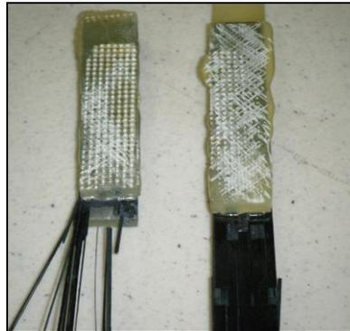
Figure 7. Continuous (*left*) and discontinuous (*right*) samples after testing. Because the glass tabs on the discontinuous samples shifted while the adhesive was curing, additional testing will be done to determine if the positioning of the glass tabs effects the tensile strength.
