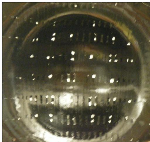
Figure 9. Back side of a (0/90) straight cut unitape hemisphere. The hemisphere is held up to a light to show the location of holes.
